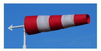
A wind sock is a type of kite used to detect wind direction and speed. It is a tapered tube of cloth held open at one end by a stiff ring.
